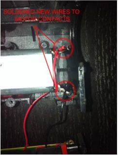
5. At this point you can put the motor back into place. You'll want to route the wires underneath the motor and you may need to cut a bit of plastic out to get the motor to re-seat properly. The wire should be routed towards the back of the feeder.
