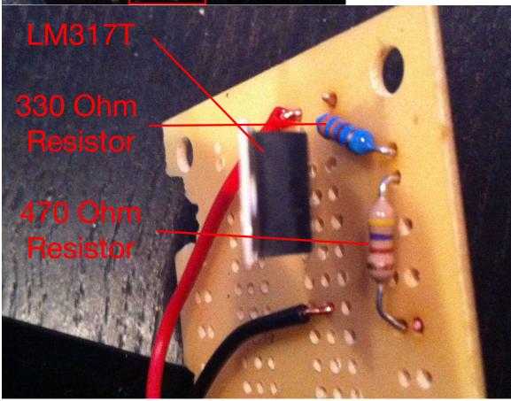
Once you have the converter and the Eheim-Mod finished, put your batteries back in the feeder. You can set the time if you like, but there is no need to. Make sure you double check the voltage coming out of your converter so you don't fry your feeder or motor.
