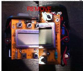
2. <u>Using a small screw driver, slide the positive battery terminal up to free it.</u>
