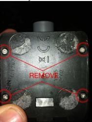
2. Remove 2 screws on either side of casing.
