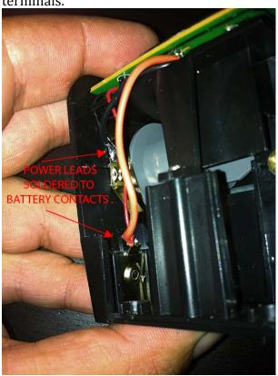
5. Route the wires underneath the circuit board.
