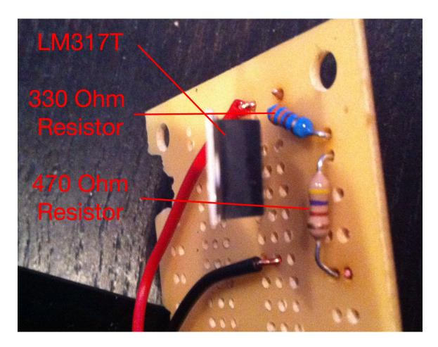
Once you have the converter and the Eheim-Mod finished connect both leads. Plug the feeder power (5-3.2V) into a power outlet, and the feeder relay (12V) into an outlet on your energy bar. You can set the time if you like, but there is no need to. Make sure you double check the voltage coming out of your converter so you don't fry your feeder or motor.
