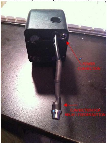
Solder to leads to the feeder button as shown in the picture. 8. FEEDER BUTTON CONTACTS PD5
