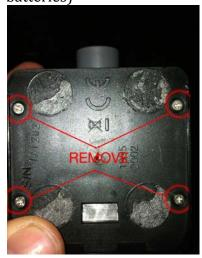
2. Remove 2 screws on either side of casing.
